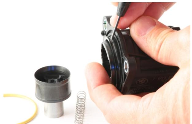
Assemble the GFB parts onto the factory solenoid body as shown in the exploded view below, making sure to use the GFB-supplied plunger spring, and the yellow o-ring removed from the factory valve. Apply some engine oil to the piston during this process. Note that regular re-lubrication is NOT required.
